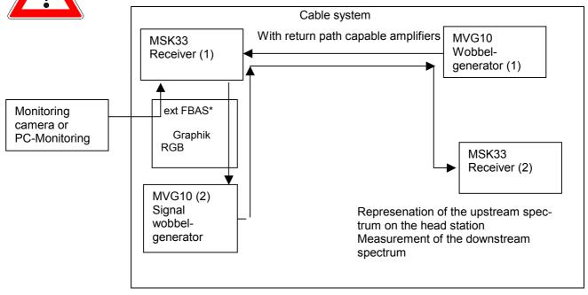
\* In case you want to additionally transmit a CVBS signal via the MVG 10 (2) in this measurement arrangement, you must change the SCART cable between MSK 33 (1) and MVG 10 (2) as follows:
